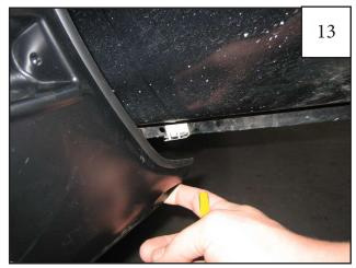
Pull back each end of flare and install assembled Clips (CL1-0008 & CL1-0010), aligning holes in clips with marks made in Step 11. The snap lock feature of the Clip should be facing outward.
