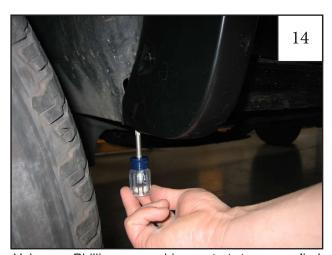
Using a Phillips screwdriver, start two supplied Screws (SW1-0049) into Clips installed in Step 13. If necessary use an awl to locate holes and adjust clips. Do not tighten. Check flare position and make sure flare fits into style line.
